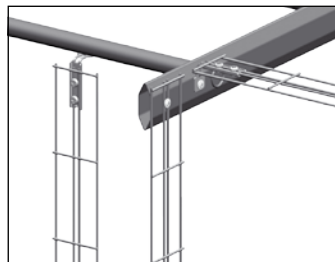
B30-I mounted onto cable ladder.
