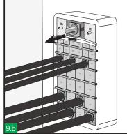
Insert the outer blocks of the endpacker. Then, untighten the compression tool and remove it.
