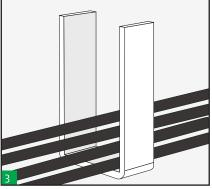
Place frame around cables. Tack weld end piece back into place. End piece should be centred in the lateral bars.
