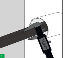
Check the inside diameter of the sleeve and the outside diameter of the cables to verify that it is within the range of selected HRST.
