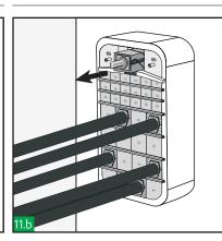
Insert the outer blocks of the endpacker. Then, untighten the compression tool and remove it.
