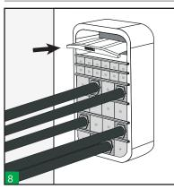
Insert the last stayplate and the compression plate before the last row of blocks (or earlier if required). Check frame packing space. Verify that the complete sealing area of this frame size (see table) will be filled with blocks.
