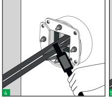
Take measures of the cables diameters and select the appropriate Hawke Tolerant blocks. Colour code will help you to select the correct ones.
