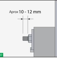
Approximately 10-12 mm of thread should protrude on each bolt.
