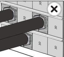
Check the correct orientation of the blocks.
