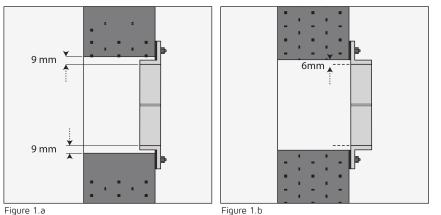
Size to fixing holes and type of fastener is to be established by the civil contractor dependent on size of frame weight and structure to which it is to be fixed. When fixing frames to concrete/ brick type structure care should be taken if using expanding type fixings as they could burst into the aperture.
