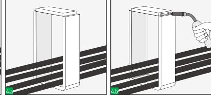
Tack weld end piece back into place. End piece should be centred in the lateral bars.
