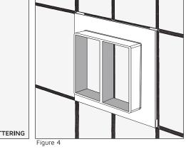
Frames and moulds require support to ensure that the correct position is maintained whilst the concrete is being poured. This may be achieved by nailing though the shuttering into the mould (if used) and fixing the frame to the rebar.
