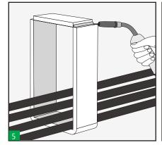
Run root fillet weld for full width of frame.
