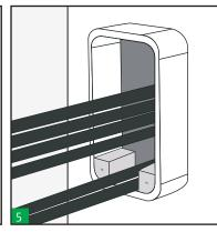
Insert HF200/R20 or HF300/ R20 round corner blocks in the bottom corners of the frame.
