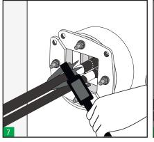
Take measures of the cables diameters and select the appropriate Hawke Tolerant Blocks.
