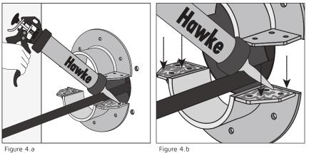
If CBO open sleeve is used, Mastic/Silicone should be applied also in all bolting areas of the removable end as showed below.
