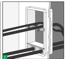
Clamp tool can be used to fix cables on the tope part of the penetration allowing an easier installation of blocks.
