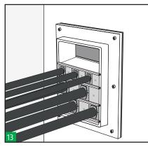
A stayplate is always inserted between each layer of blocks.
