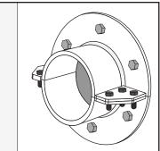
Check that Hawke Sleeve has been used in the in stallation, that it has been properly installed (welded/bolted) and that is has not mechanical or corrosion damage.
