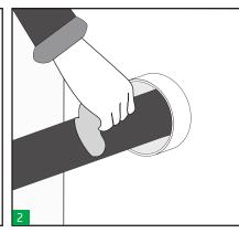
Make sure the pipe is properly centred in the sleeve. Make sure the sleeve and the cable/pipe are clean.
