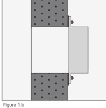
Size to fixing holes and type of fastener is to be established by the civil contractor dependent on size of sleeve weight and structure to which it is to be fixed.
