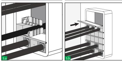
Begin packing the frame. Colour code will help you to install the blocks correctly. A stayplate is always inserted between each layer of blocks. Blocks should not protrude out of the stayplates retaining lips.
