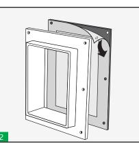
Remove the protection and stick the gasket on the aluminium frame.
