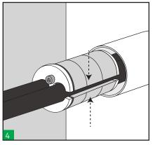
Open the HRST and install around the cables.
