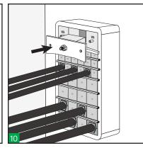
Insert the centre piece of the endpacker along with the front plate.
