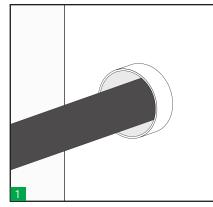
Check the inside diameter of the sleeve and the outside diameter of the cable/pipe to verify that it is within the range of selected HRST. Hawke HRST colour code will help for a correct selection.
