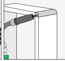
Clean both ends of weld/frame and spot weld them to ensure seal. Weld should not penetrate inside the corner of the frame.
