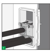
Clamp Tool can be used to fix blocks in their place when the transit installation is not completely finished.
