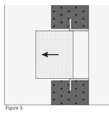
When all shuttering and other formwork has been removed, the polystyrene mould must be removed prior to electrical installation.
