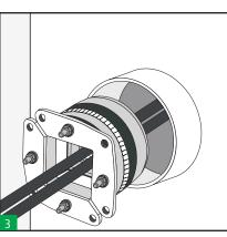
Insert the round transit frame completely in the sleeve around the cables and open the two front plates. (HRTO30,HRTO40&HRTO50 front plates are fixed). No lubricant should be applied to the aperture or outside of the frame.
