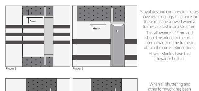
This allowance is 12mm and should be added to the total internal width of the frame to obtain the correct dimensions. Hawke Moulds have this
