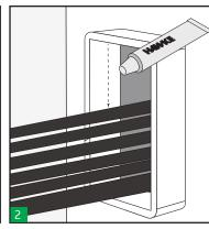
Lubricate the inside of the frame. Ensure the corners are well lubricated.
