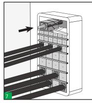
Pack the last row between the last stayplate and the compression plate. Insert the compression tool on the top, in the centre of the compression plate.
