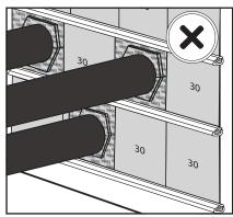
Check that there are a stayplate between each row of blocks and there are not stayplate between the bottom row of blocks and the frame.
