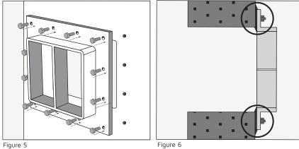
The frame can now be placed over its fixings and fasteners tightened to clamp the frame to the wall/floor.
