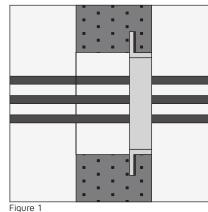
The frame can be casted directly into a wall or floor.
