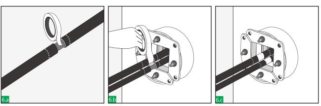
Using copper tape provided tightly wrap around the exposed screen until the cable outer diameter is regained. Repeat these steps for all cables.
