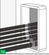
Cut and remove cable sheath between two central marks, to expose the cables conductive screen.
