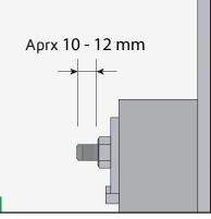
Approximately 10-12 mm of thread should protrude on each bolt to ensure the sealing.
