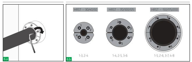
Tighten the bolts. Tightening must be done in one revolution step for each bolt following next sequence until the system is enough compressed to seal the cable/pipe.
