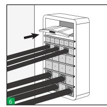
Insert the last stayplate and the compression plate before the last row of blocks (or earlier if required).Check frame packing space. Verify that the complete sealing area of this frame size (see table) will be filled with blocks.
