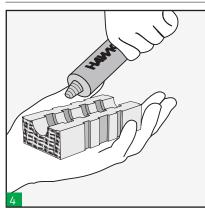
Lubricate all the insert and blank blocks using Hawke lubricant.
