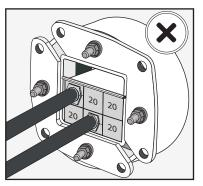
Check that Hawke Sleeve has been used in the installation, that it has been properly installed (welded/bolted) and that is has not mechanical or corrosion damage.
