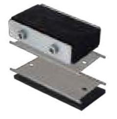
Hawke CSDM Compression system is used in H-DM frames to compress and seal the installation of cables and DM modules. It includes the endpacker unit, 5mm filler strip and two stayplates. The 5mm filler strip can be installed as either the top or bottom row of blocks within a H-DM aperture.
