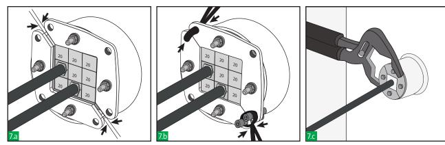
Slide the two front plates together and keep it fixed. Ensure all the blocks are located inside the front retaining lip. For an easier installation, cable ties , bolts or adjustable pliers can be used to close this plates.
