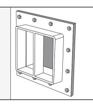
Check that Hawke Frame has been used in the installation, that it has been properly installed (welded/bolted)and that it has not mechanical or corrosion damage.
