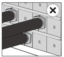
Check the correct orientation of the blocks.
