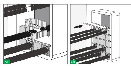
Begin packing the frame from the bottom to the top. A stayplate is always inserted between each layer of blocks. Blocks should not protrude out of the stayplates retaining lips. Ensure when fitting cables into blocks that copper tape on blocks and cable align. Marks in the cable will help to guarantee it.
