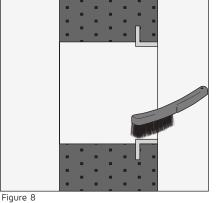
When all shuttering and other formwork has been removed, the polystyrene mould must be removed prior to electrical installation.
