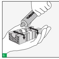
Very slightly lubricate all the insert and blank blocks using Hawke lubricant taking care not contaminate the copper on blocks and cables.
