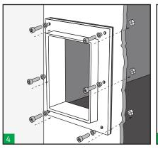
Insert bolts washers and nuts to the frame/ enclosure.
