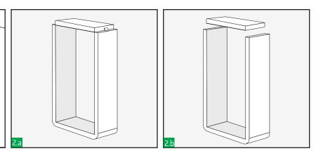
Break tack welds and remove end piece from the frame.
