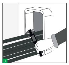
Take measures of the cables diameters and select the appropriate Hawke Tolerant blocks. Colour code will help you to select the correct ones.
