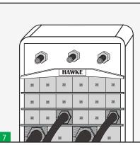
Tighten the nuts on the endpacker alternately following the above sequence to compress and complete the seal. Use a ratchet spanner for an easier installation. Approximately 10-12 mm of thread should protrude on each bolt to ensure the sealing.
