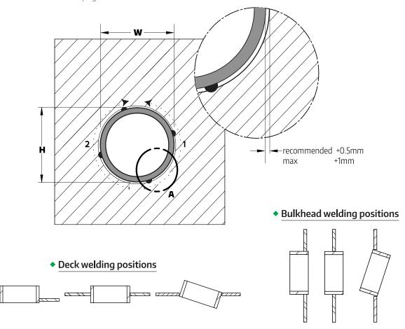
2. Tack weld on the front side, centring the frame onto the cut-out hole:
