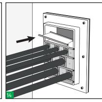
Insert the last stayplate before the last row of blocks (or earlier if required). Verify that the complete sealing area of this frame size (see table) will be filled with blocks. Note: 5mm strip supplied with the compression system should be not considered as part of the sealing area.
