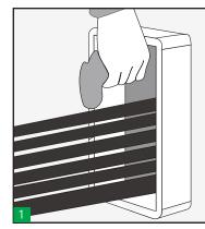
Make sure the frame is clean, then pull cables or pipes through, placing the largest at the bottom. (Note: Use open ended frame to fit around existing cables/pipes)
