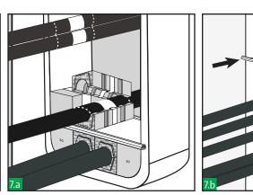
Begin packing the frame from the bottom to the top. A stayplate is always inserted between each layer of blocks. Blocks should not protrude out of the stayplates retaining lips. Ensure when fitting cables into blocks that copper tape on blocks and cable align. Marks in the cable will help to guarantee it.
