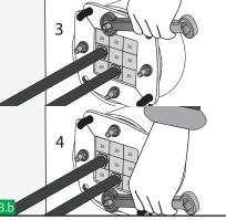
Tighten the nuts approximately 2mm each time following alternate tightening sequence, applying equal pressure to both plates. A minimum of 10 mm of thread should protrude on each bolt. Use a ratchet spanner for an easier installation.
