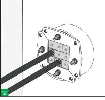
Tighten the nuts approximately 2mm each time following alternate tightening sequence, applying equal pressure to both plates. A minimum of 10 mm of thread should protrude on each bolt. Use a ratchet spanner for an easier installation.
