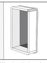
Weld frame in position in accordance with Rectangular frame HMX welding instructions and seal the frame in accordance to rectangular system installation guide.
