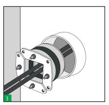
Insert the round transit frame completely in the sleeve/aperture around the cables. No lubricant should be applied to the aperture or outside of the frame. If close version of the Round Transit(HRT) is used, it should be installed previously to pull the cables/ pipes through the sleeve or aperture.
