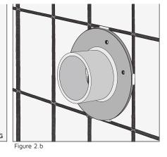
Sleeves and moulds require support to ensure that the correct position is maintained whilst the concrete is being poured. This may be achieved by nailing though the shuttering into the mould (if used) and fixing the frame to the rebar.
