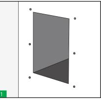
Cut a rectangular opening for the frame according to H-DH frame size to be used.(See table).
