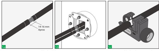
Cut and remove cable sheath between two central marks, to expose the cables conductive screen.
