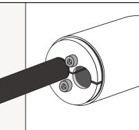
Check that every not occupied HRST holes are plugged with Hawke HRST plugs.
