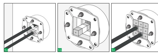
Begin packing the transit frame starting at the bottom and finishing at the top. Ensure that the blocks are pushed firmly against the rear retaining lip. Verify that the complete sealing area of this frame size (see table) is filled with blocks.
