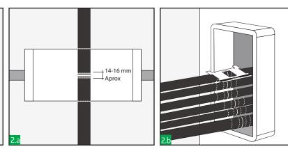
Mark each cable in the centre of the frame and 7-8mm either side of this point. Also, recommendable to mark the cable in both ends of the frame. EMC marking tool could help you to reduce time and ensure a correct marking.
