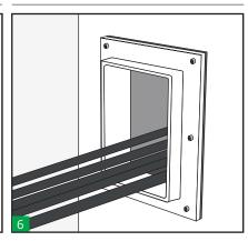
Pull cables or pipes through, placing the largest at the bottom.
