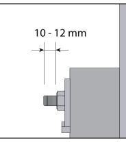
Approximately 10-12 mm of thread should protrude on each bolt to ensure the sealing.
