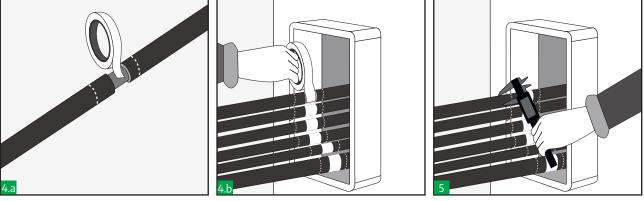
Take measures of cables diameters and select the appropriate Hawke tolerant blocks.
