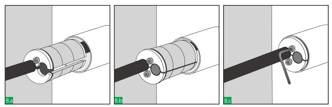
In case of any HRST hole are not occupied by cables always complete with Hawke HRST plugs.
