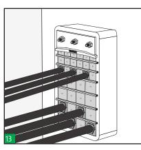
Make a visual inspection of the transit. Hawke's unique colour coding system enables the installation to be visually inspected after completion and ensures correct matching of the block halves.
