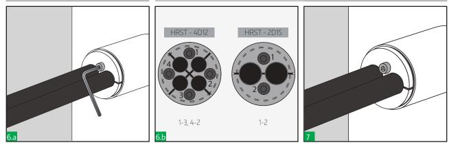
Tighten the bolts. Tightening must be done in one revolution step for each bolt following next sequence until the system is enough compressed to seal the cables.
