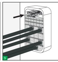
Pack the last row between the last stayplate and the compression plate. Insert the compression tool on the top, in the centre of the compression plate.
