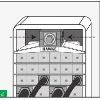
Compression tool must be introduced centred in the frame both in width and depth since otherwise the compression of the system would not be balanced so that to be able to introduce the lateral pieces of the endpacker t it would be necessary to over tighten the tool and it could be damaged.
