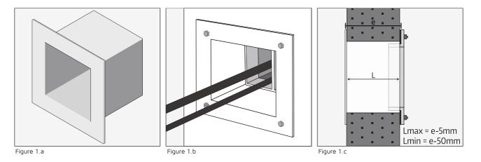
These maintain the openings through the wall and floors and add the finished appearance of the installation. It should be noted that the backing plates do not add to the fire resistance of a transit and should be not used to stop fire spread in cavity walls.
