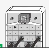
Insert the outer blocks of the endpacker. Then, untighten the compression tool and remove it.
