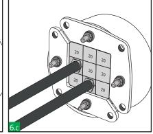
Begin packing the transit frame starting at the bottom and finishing at the top. Ensure that the blocks are pushed firmly against the rear retaining lip. Verify that the complete sealing area of this frame size (see table) is filled with blocks.
