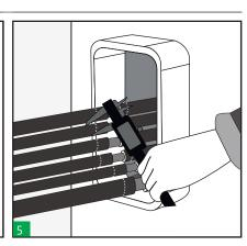
Take measures of cables diameters and select the appropriate Hawke tolerant blocks. HTS-EN-AI008-Rev03-10/19
