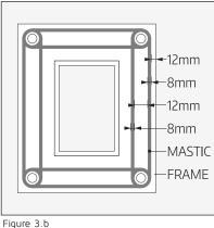
Cut nozzle on Mastic/Silicone tube to produce a bead diameter of approximately 8mm.
