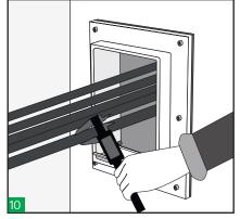
Take measures of the cables diameter with a calibre and select the appropriate Hawke tolerant blocks. Colour code will help you to select the correct ones. Only use H-DM black blocks.
