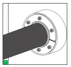
Make a visual inspection of the transit. HRST (colour code) selected match the pipe and sleeve installed, HRST is completely inserted into the sleeve, does not exist gaps between HRST and the cable/pipe.
