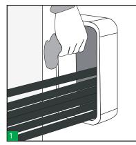
Make sure the frame is clean, then pull cables or pipes through, placing the largest at the bottom. (Note: Use open ended frame to fit around existing cables/pipes)
