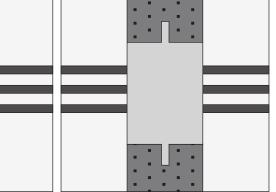
The sleeve can be casted directly into a wall or floor.
