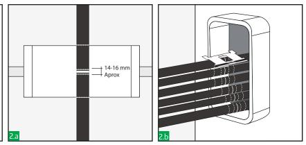
Mark each cable in the centre of the frame and 7-8mm either side of this point. Also, recommendable to mark the cable in both ends of the frame. EMC marking tool could help you to reduce time and ensure a correct marking.
