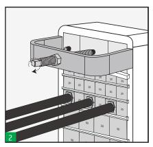
Remove endpacker nuts and front plate.
